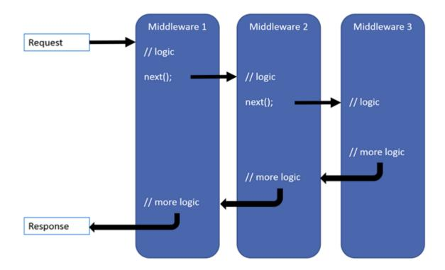
The preceding diagram lacks a concept of lifecycle events. This concept is foundational to how ASP.NET Web Forms requests are handled. This system makes it easier to reason about what process is occurring and allows middleware to be inserted at any point. Middleware executes in the order in which it's added to the request pipeline. They're also added in code instead of configuration files, usually in *Startup.cs*.
