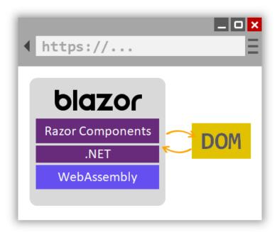
Blazor WebAssembly apps run purely client-side. Such apps can be deployed to static site hosting solutions like GitHub Pages or Azure Static Website Hosting. .NET isn't required on the server at all. Deep linking to parts of the app typically requires a routing solution on the server. The routing solution redirects requests to the root of the app. For example, this redirection can be handled using URL rewrite rules in IIS.
